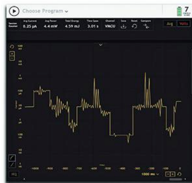
Silicon Labs’ energyAware Profiler tracks power utilization, in addition to power modes and peripheral status.
